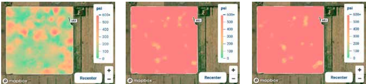
South field compaction maps at 3", 12" and 18" depth respectively.
